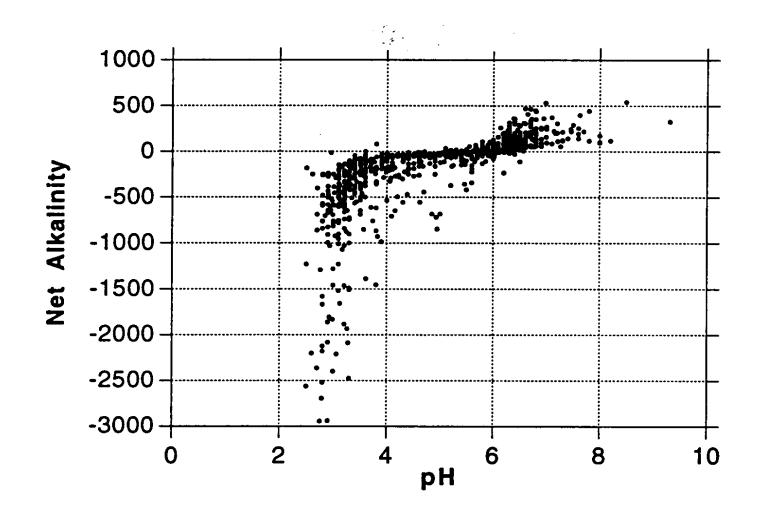
Figure 1.2, Graph C, net alkalinity vs. pH, page 1-5, of Coal Mine Drainage Prediction and Pollution Prevention in PA
