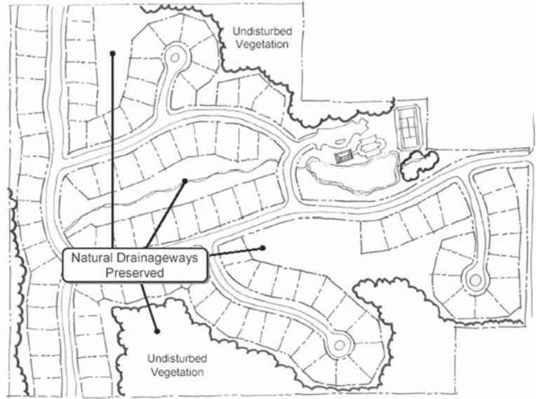
Figure 5.3-1. Protecting natural drainage features
