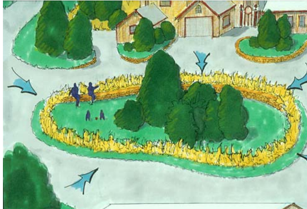
Figure 5.3-6. Natural surface depressions can temporarily store stormwater.
