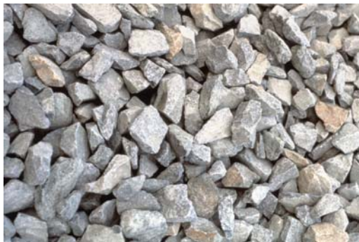
Figure 6.1-27 The uniformly-graded stone must be washed and clean.
