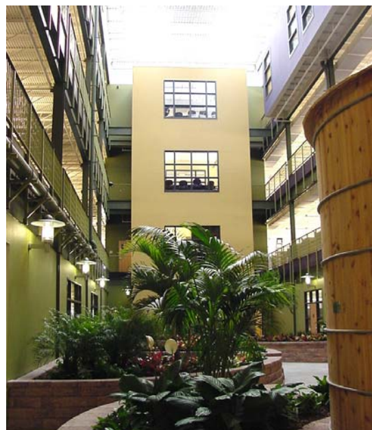
Figure 7-17. First floor atrium w/ 5,000-gallon wooden cistern on right (Source: PA DEP Southeast home page).
