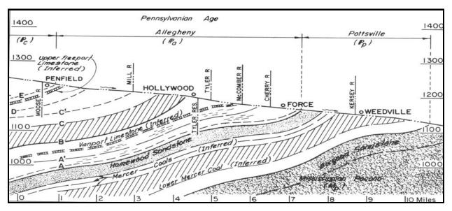
Figure 6. Profile along the axis of the Caledonia Syncline showing the plunge in the opposite direction of the stream flow (Source: Berger).
