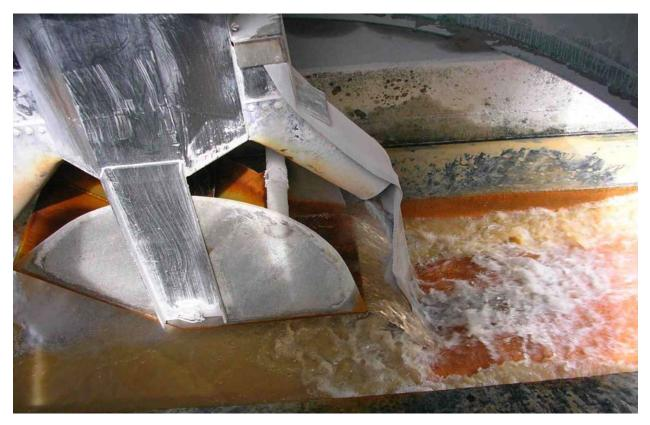
Figure 21. Tipping bucket mechanism dispensing lime to neutralize the highly acidic discharge.
