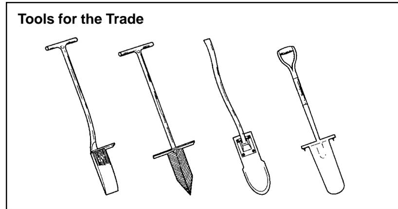
Figure 11: Tree-planting tools (left to right): planting bar, a pointed planting bar for stony soils, the Rindi grub-hoe (L-shaped) for making straight-sided holes, and a tile spade planting shovel for digging deep holes for large planting stock. (Source: The Practice of Silviculture, Smith, 1986).
