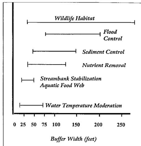
Figure 4. Range of minimum widths for meeting specific buffer objectives.
