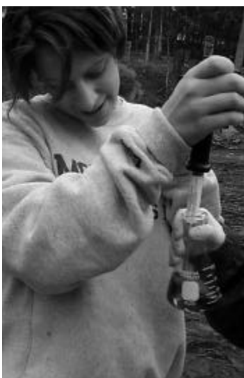
Keystone College participant titrates a water sample in an erlenmeyer flask.
