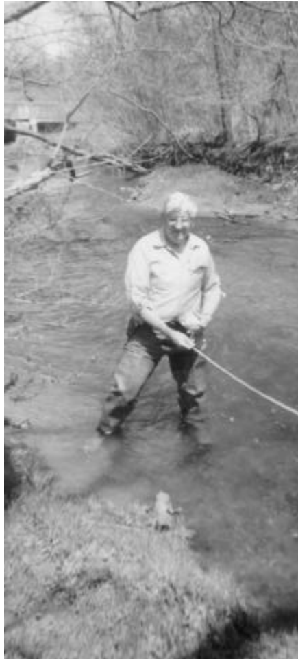
Amel Johnson measures stream width and calculates flow rate.
