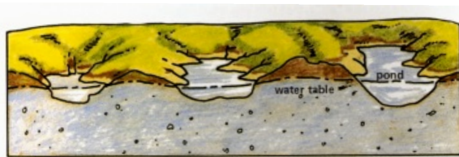
Land surfaces dipping below the water table will create ponds or lakes.
