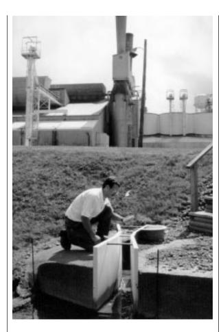
PPG Industries Inc. works: Meadwille, PA. Plant Environmental Engineer checking the pH of discharge water from plant operations.
