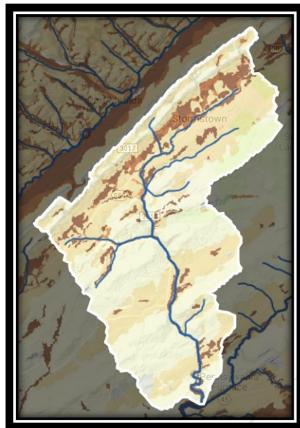
Figure 4a. and 4b., Comparison of soil distribution in Halfmoon Creek and Beaver Branch (tan-A-slow infiltration, yellow-B-moderate, orange-C-slow, red-D-very slow infiltration)
